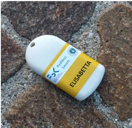
Figure 8 Proximity device that all children taking part in the PBS initiative receive to allow the automated registration of their attendance.
